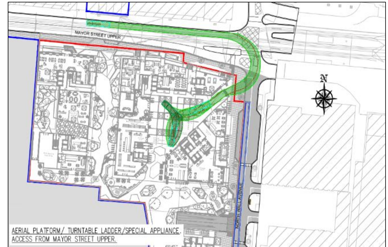
Figure 4.3: Extract of Dwg. No. R064-210, 'Autotrack – Ground Level – Fire Tender', Rev. E. Source: CS Consulting, January 2021. Cropped by TPA, January 2021.
